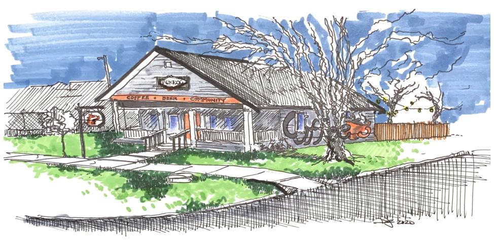
Proposed conceptual design for street front exterior illustrating signage options integrated with landscape and building elements as well as a "supergraphic" mural hand painted on building face. Note script and illustration are intentionally not confined by existing window placement. Post sign at sidewalk allows for a crafted pedestrian scale opportunity for logo placement and building numbers.
