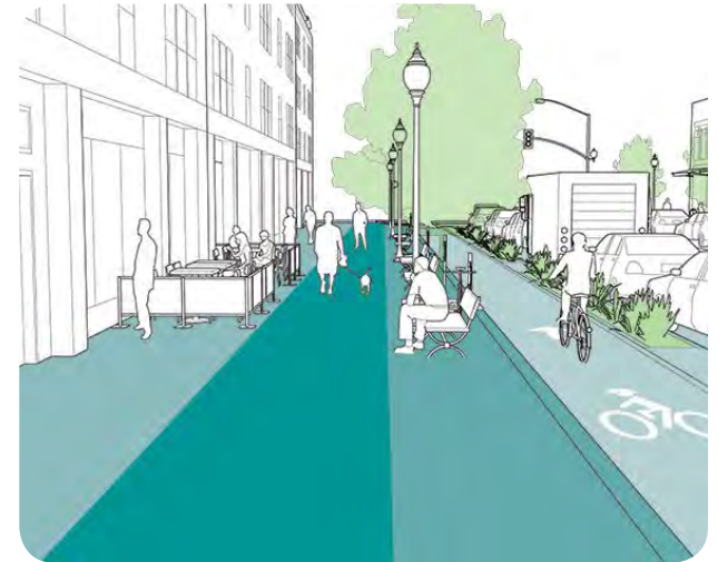
Above: This illustration identifies the integration of 15' sidewalks with the street trees, furniture, planting strips and the separation from bike lane to road. Below: Furnishings, signage, and other moveable elements should be placed to maintain a clear path for pedestrians.
